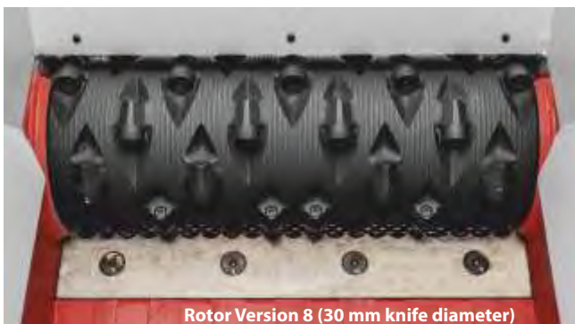
Rotor Version 8 (30 mm knife diameter)
