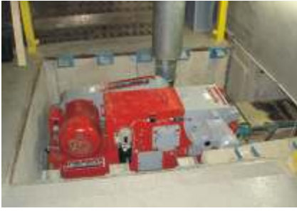
Shredding wood waste from a plate saw with an RHZ 400 S horizontal shredder set up below ground
