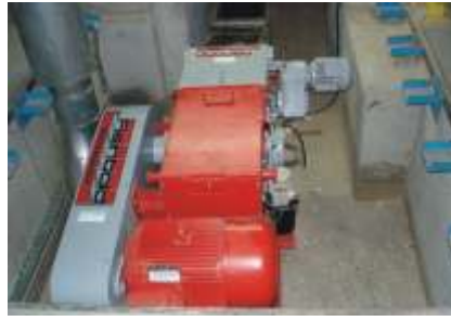
Shredding wood waste from a plate saw with an RHZ 400 S horizontal shredder set up below ground
