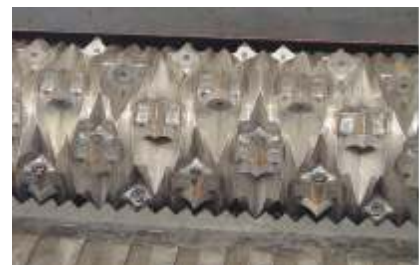
Concave cutting heads can be turned up to 4 times.
