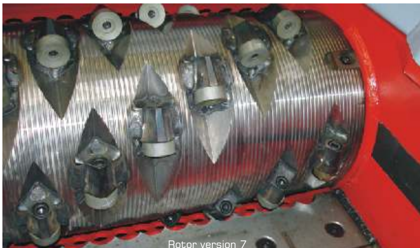
Concave cutting heads can be turned up to 4 times.
